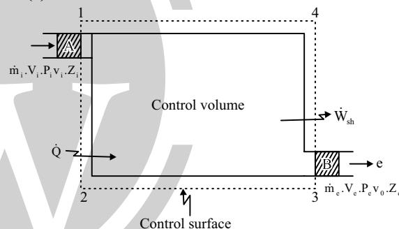
A control volume is a specified region in space through which mass may flow, and it is used for analyzing fluid flow systems like turbines, compressors, and pumps. The control volume approach helps in understanding the energy and mass transfer within a defined boundary.
