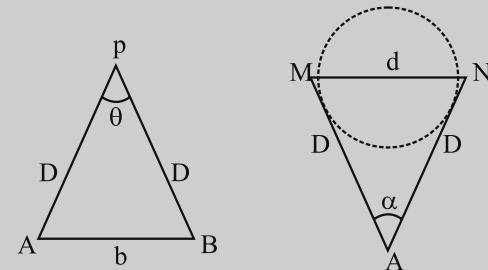
The angle  $\theta$  between the two directions along which the planet is viewed at the two points is measured, which is called parallax angle or parallactic angle. Since  $\theta$  is small,  $AB$  can be considered as an arc of length of a circle with center at  $P$  and the distance  $D$  as radius
