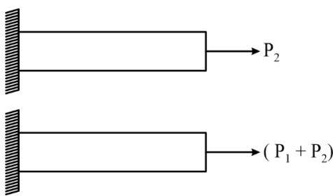
If  $U$  is the strain energy stored in the same bar when subjected to an axial tensile force  $(P_1 + P_2)$ , the correct relationship is
