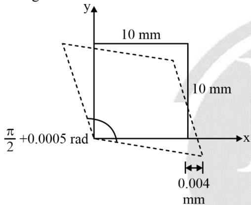
If the shear strain  $\gamma_{xy}$ , at this point is expressed as  $0.001 k$  (in rad), the value of  $k$  is
