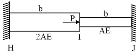
To make the axial force in rod HI equal to zero, the value of the external force  $P$  (in N) is \_\_\_\_\_. (Rounded off to the nearest integer)
