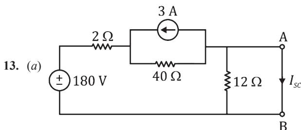
To find Norton's current, short circuit the terminal A and B and find  $I_{SC}$
