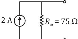
$$I = \frac{V_{OC}}{R_{in}} = \frac{150}{75} = 2 \text{ A}$$
