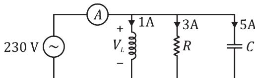
Here ammeter reading will be phasor sum of  $I_R$ ,  $I_L$  and  $I_C$
