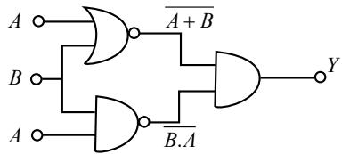
& the output of NOR gate is  $\overline{A + B}$  the output of NAND gate is  $\overline{AB}$
